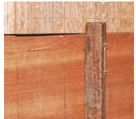
▲ Pic.13 Marking the line, Jason needed to hand cut to for the rest of the middle rail
